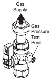
Ensure that this inlet pressure can be obtained with all other gas appliances in the property working at maximum.
